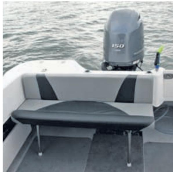
A collapsible rear seat makes a lot of sense in a fishing boat. When folded down for serious work the back rest makes a handy bolster as well.
