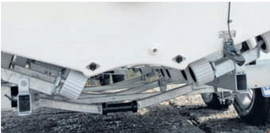
The one item that really sets this craft apart is the Hydralift hull design. Note the large tunnel section with its pair of keels.
